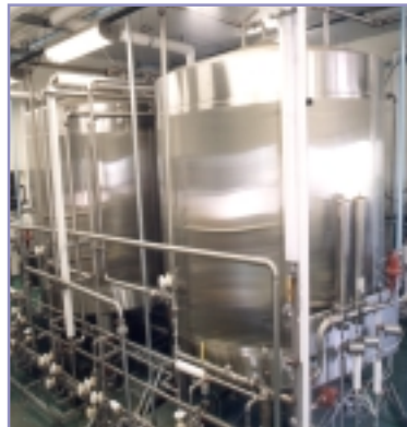
Aseptic Tank -keeps product sterile prior to packaging
