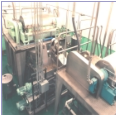
Decanter -separates the liquid from the solids
