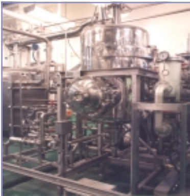
Sterilization -After blending, product is pumped through a sterilizer
